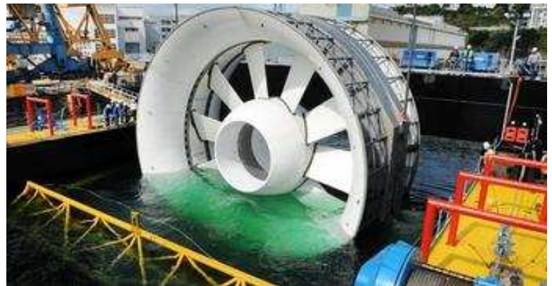
Photographed in Brest is OpenHydro's latest 16m tidal turbine
